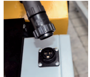
Motor is connected to the electronic panel with a snap-on connector
