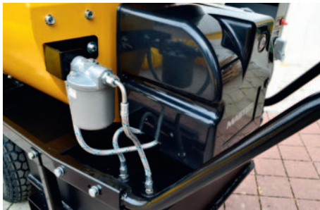
Fuel filter is outside. Fuel pre-heater is inside, within the combustion head
