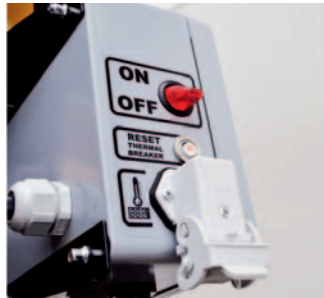
Control panel including on/off switch with LED
